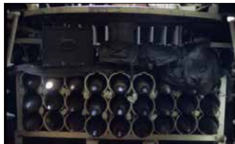
The ammo rack under the 105 Howitzer Mount that took a B-40 hit through two empty tubes.
